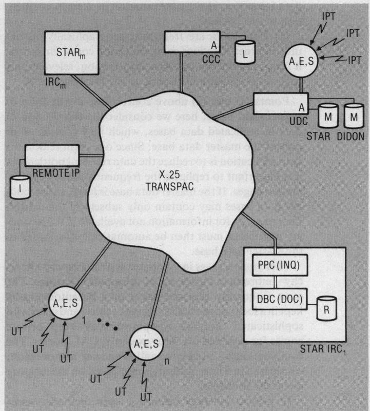
Figure 5. Distributed Videotex system used in Antiope.
