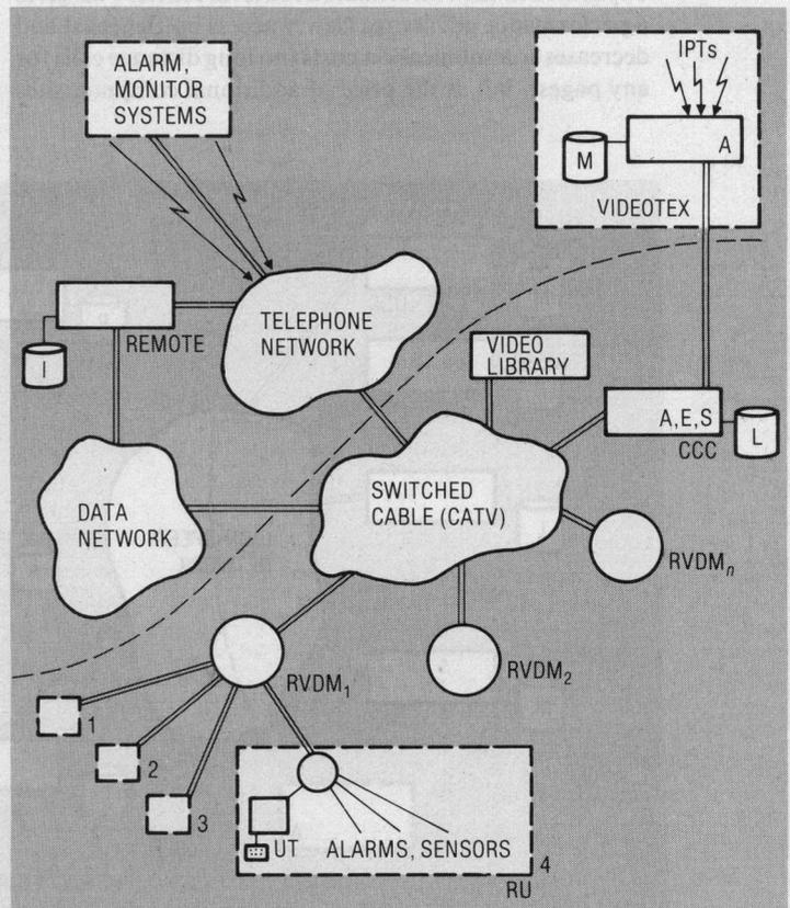
Figure 6. A multiservice, distributed processing system such as Omnitel.
